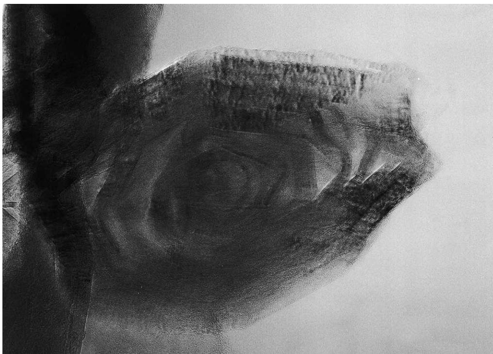
Fig. 20. TEM picture of MCMB heat-treated at 2750 °C (20 nm=10 nm).
